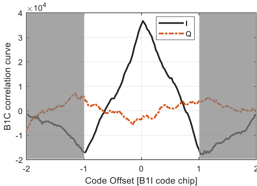
Figure 16: The correlation function curve of the B1C pilot BOC(1,1) component with proposed tracking method
